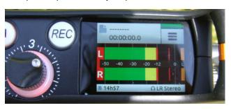
headphone knob is also used for text selection or to audio scrub during playback. The fader knobs are surrounded by a variable LED which shows increasingly green when there is a good signal and red when peaking - so you have a very clear indication about levels without even looking at the meters on screen. I found the touch screen a bit fiddly to use at first due to the small size of the button areas but I soon got used to it. Fortunately the menu logic is clear and easy to follow.
