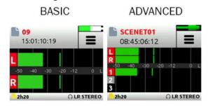
In Advanced mode you can record to individual tracks at pre-fade level, which you set up on the menu screen and adjust with the multi function headphone knob - and of course you can record a stereo output at the same time. SoundDevices say that the inputs are so clean and quiet that you can record at very low levels and boost the signal afterwards without introducing noticeable noise, although I always find it comforting to see a decent signal on the meters! There is also a useful Aux
