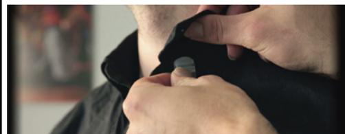
The RØDE invisLav is designed to aid the concealing of the Lavalier and smartLav microphones.
