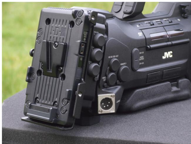
The handle incorporates a very solid shoe mount at the front and also has two 1/4 inch threaded screw holes for mounting heavier gear on top. For tripod mounting the camcorder comes fitted with the industry standard 'Sony type' V shoe and stud mount. You will of course need to buy a rather expensive quick release tripod plate to bridge the shoulder pad if you need to use these shoes to mount the camcorder properly balanced on a tripod.
